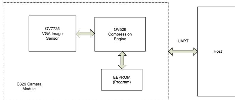
Figure 5: Camera block diagram
