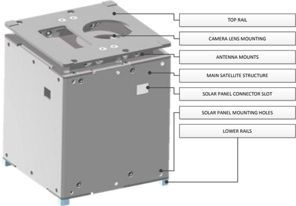
Figure 3: Cube satellite structure
