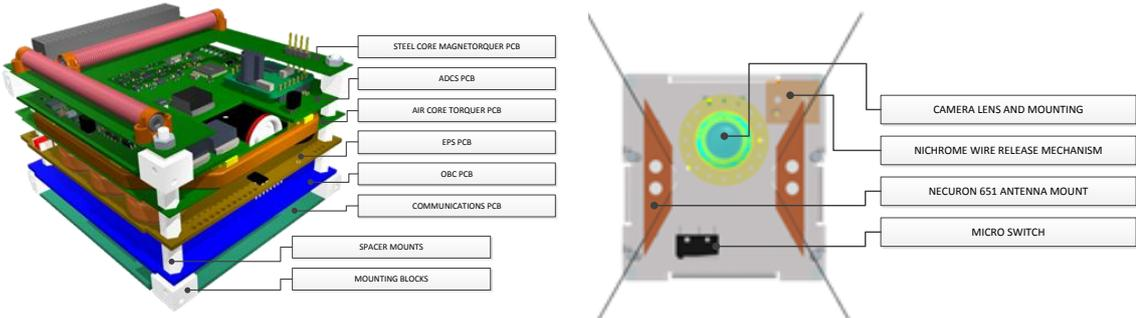
Figure 4: Satellite PCB (left) and antenna deployment system / camera mount (right)
